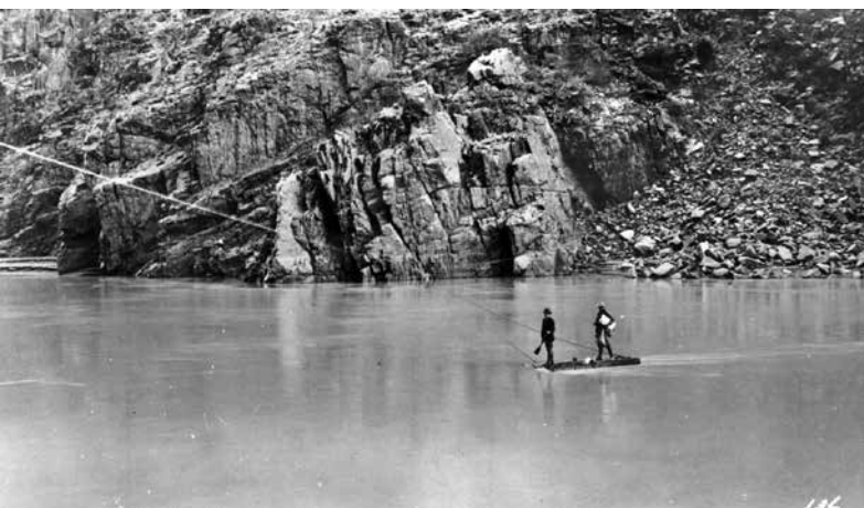
A raft attached to a crossing rope by pulley. The current did the 'heavy' work. [View toward the south side of the river. Twenty or more oil cans provided buoyancy for the raft.] GCNP Museum Collection.
